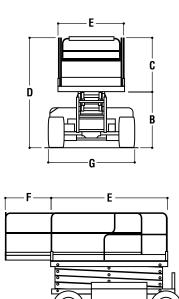
5 ft 9 in. (1.75 m) G. Overall Width H. Overall Length (no outriggers) 8 ft 9 in. (2.67 m) I. Wheelbase 6 ft 6 in. (1.98 m) J. Ground Clearance 8 in. (20 cm)
