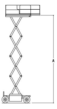
A. Platform Height Elevated 26 ft (7.92 m) B. Platform Height Lowered 4 ft 1.5 in. (1.26 m) C. Platform Railing Height 3 ft 7.5 in. (1.1 m) D. Overall Height 7 ft 9.5 in. (2.37 m) E. Platform Size 65 x 102 in. (1.65 x 2.59 m) F. Platform Extension 4 ft (1.22 m)
